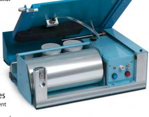
The imaging film and developers are safely located under the vacuum bed for compact transportation. ESDA®-Lite is quickly operational by simply attaching the imaging film roll onto the locating
